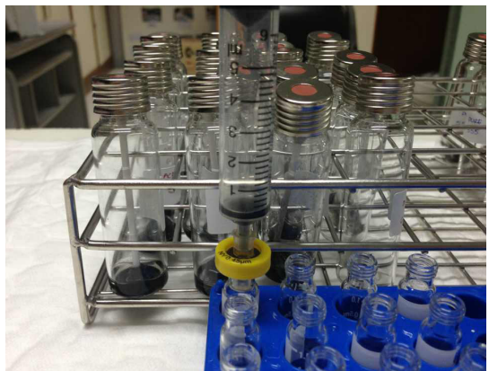
Figure 4. Solvent extraction method with syringe filtered
