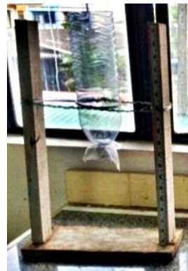
Figure 1. The water flow rate tester
