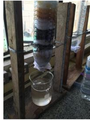
Figure 2. The filter material in flow rate tester
