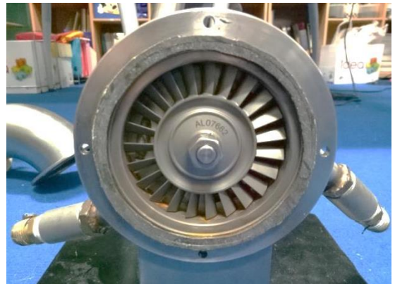
Figure 1. Reaction steam turbine
