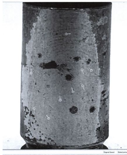
Figure 2. Latent fingerprints that appear on a 9 mm bullet by Perma blue over 3 hours.
