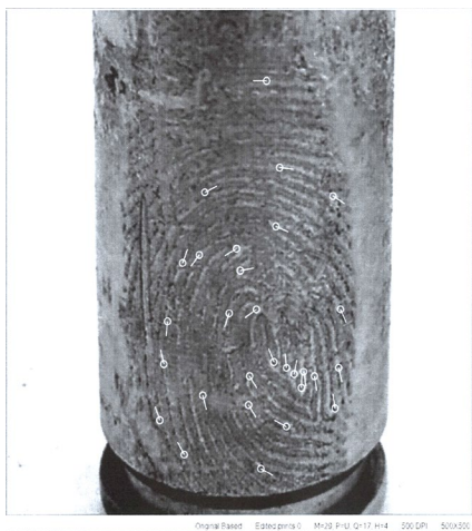
Figure 1. Latent fingerprints that appear on a 9 mm bullet by Small Particle Reagent over 3 hours.
