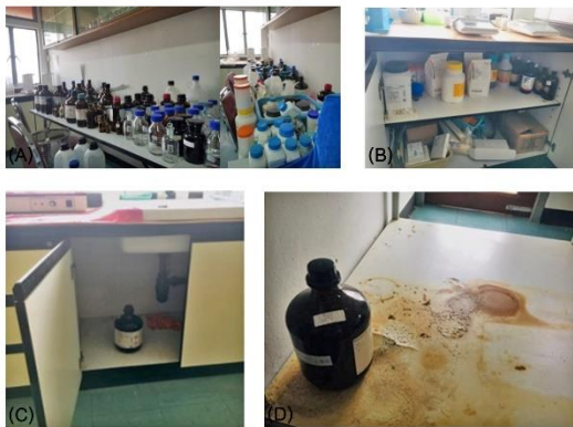
Figure 4. (A) The untidiness and mismanagement of chemical storage, (B) The storage of liquid and solid chemical together, (C) The storage of acid chemical under the sink and (D) The storage of liquid chemical without tray (before the implementation)
