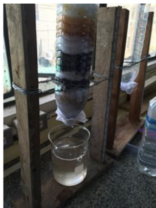
Figure 2. The filter material in flow rate tester
